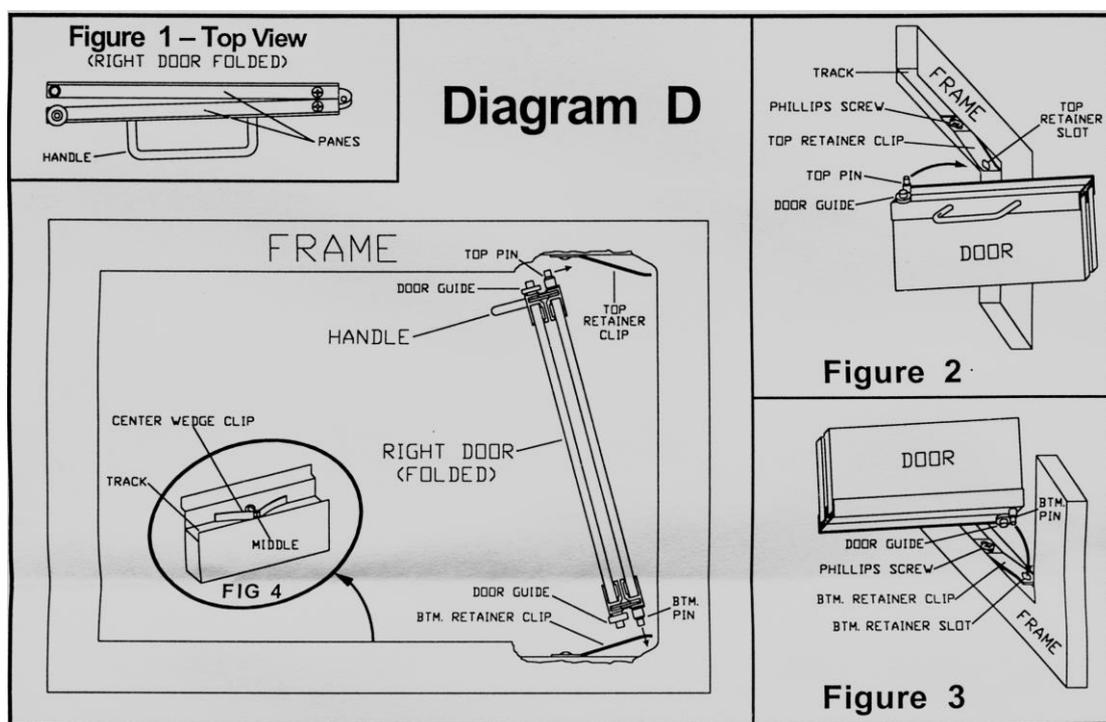
Insert the doors as per the diagram above. Please be sure to fit the frame square and vertical as this will improve the opening and closing of the doors. If you have any queries with regards to fitting please phone us. 01452 830662.
